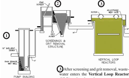
1) Flow enters the raw sewage wet-well where it is pumped by three **Raw Sewage Pumps** equipped with variable-speed drives. Two pumps have a combined capacity of over 3 MGD, with the third pump as standby. The raw sewage **Flow Meter** measures and totalizes the pumped flow.
